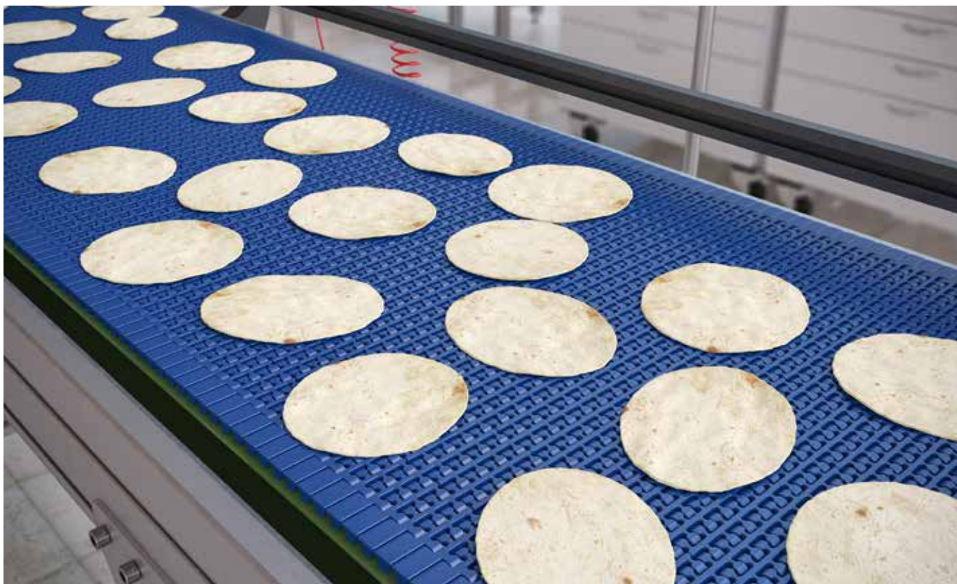
Conveyor equipped with Rexnord 596 Series KleanTop Belt.
