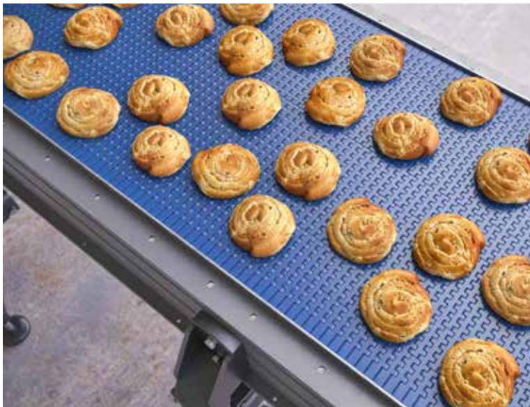
Conveyor equipped with Rexnord 595 Series KleanTop Belt.
