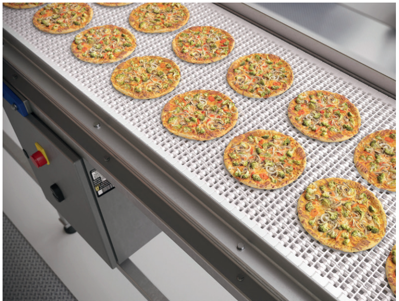
Conveyor equipped with Rexnord 1096 Series KleanTop Belt.
