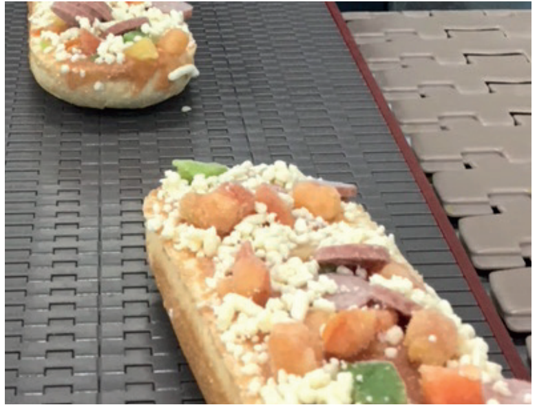
Conveyor equipped with Rexnord 395 Series KleanTop Belt.
